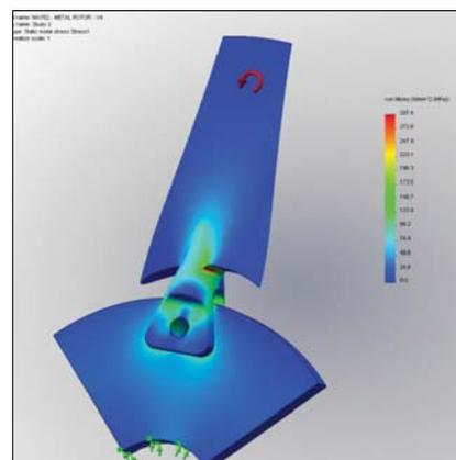
**ABOVE** Structural analysis of the cast steel rotor blades to ensure greater fatigue life and low stresses in the final assembly
