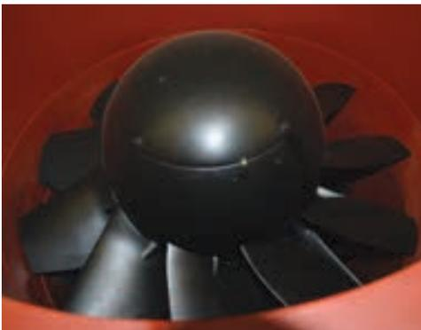
*For the impellers on the axial vane fans EN19 steel proved to have better impact resistance, but composite cone and stator vanes have been retained.*
