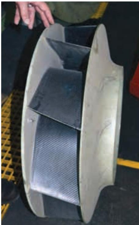
*MechCaL's carbon fibre centrifugal fans for mobile haul trucks are 60% lighter, costs less, and have proved to be 16% more aerodynamically efficient than traditional equivalents.*
