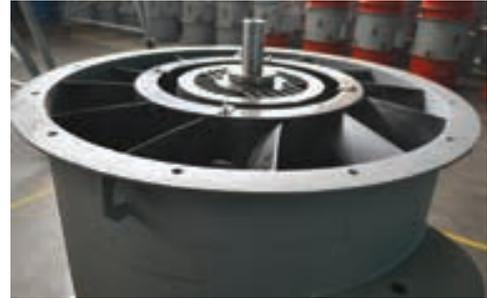
*The use of composites for the stator exit vanes allows for more complex and smoother surfaces, reducing losses and improving efficiency.*
