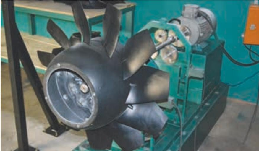
*MechCaL fans are statically and dynamically balanced. The individual blades are first weighed and a proprietary software programme sequences the placement of blades to achieve best possible static balance. An automatic dynamic balancing system is then used to identify where additional weights need to be added.*
