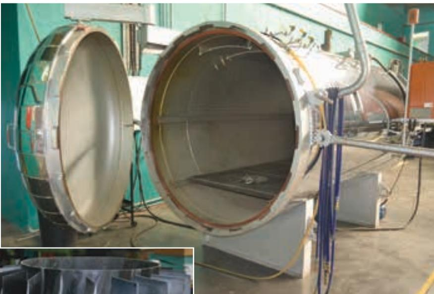
**Above:** MechCaL's 6,0 bar autoclave for curing composite components.
